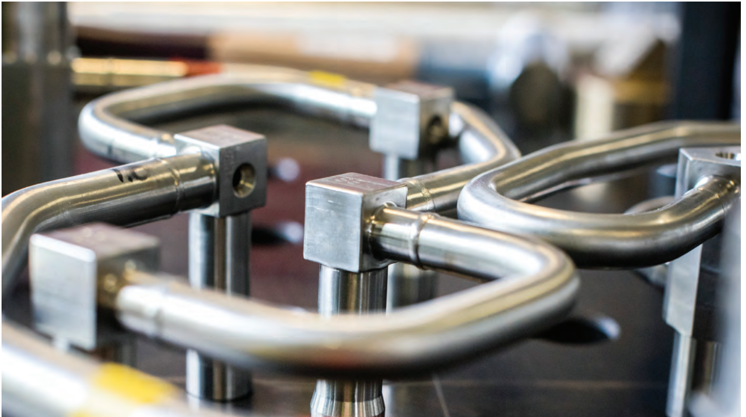
Piping with welded / brazed fittings
